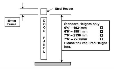
NOTE- No clearance between side frame & brickwork has been allowed for.
